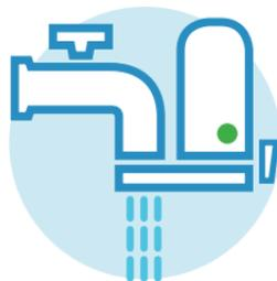
Lever in **OFF** position. **Unfiltered water** flows under faucet.
